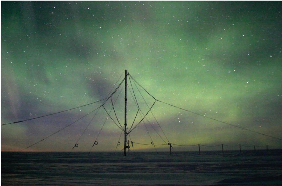
Figure 1. Loop Antenna, British Antarctic Survey Base Halley. Photo courtesy of Jeff A. Cohen from AARDVARK website.
