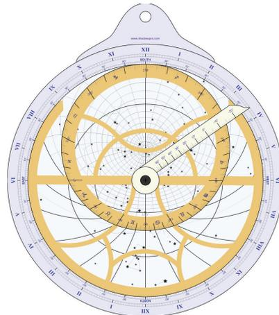
Figure 3. Modern day planispheric astrolabe designed for the latitude of Varese (Italy), drawn by the *Shadows Pro* shareware. Printable on paper.
