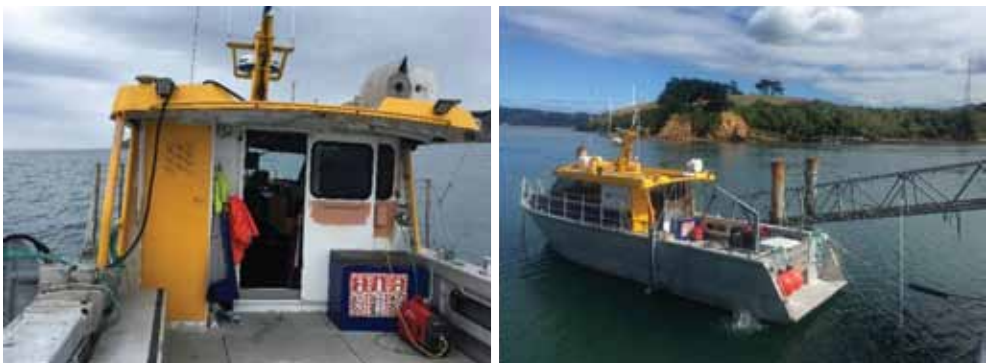
Figure 1. (L) R/V Beryl Brewin surveying coastal Otago with multibeam echo sounder equipment installed on a pole over the port side and on the roof. (R) R/V Beryl Brewin moored at Portobello Marine Lab. Photographs: E Tidey.
