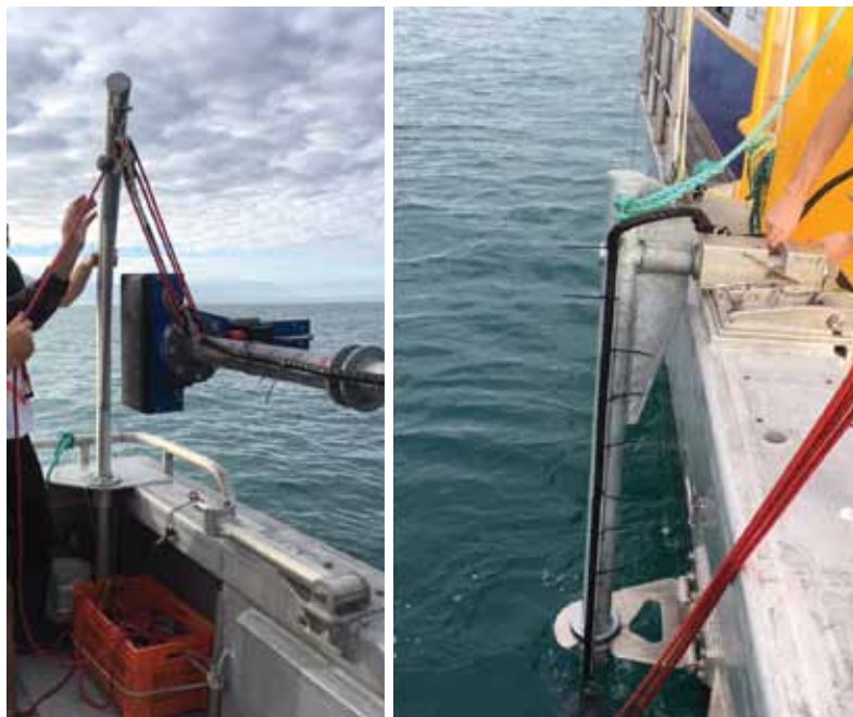
Figure 3. (L) R2 Sonic 2026 multibeam echo sounder on a pole mount. As well as acoustic transmit and receive arrays mounted at 90°, the head holds a motion sensor and sound velocity probe to correct measurements made in the dynamic sea environment. (R) Equipment deployed over the port side of the vessel; the relationship of the submerged gear and the topside positioning system must be accurately measured. Photographs: E Tidey.
