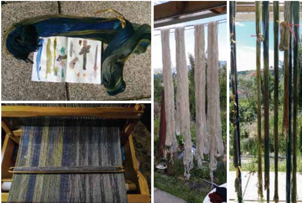
Figure 1. Dyed warp and workbook used to develop dye palette. Figure 2. Weaving in progress. Figure 3. Skeins ready for first tie-offs. Figure 4 Dyeing in progress, with last tie-offs.
