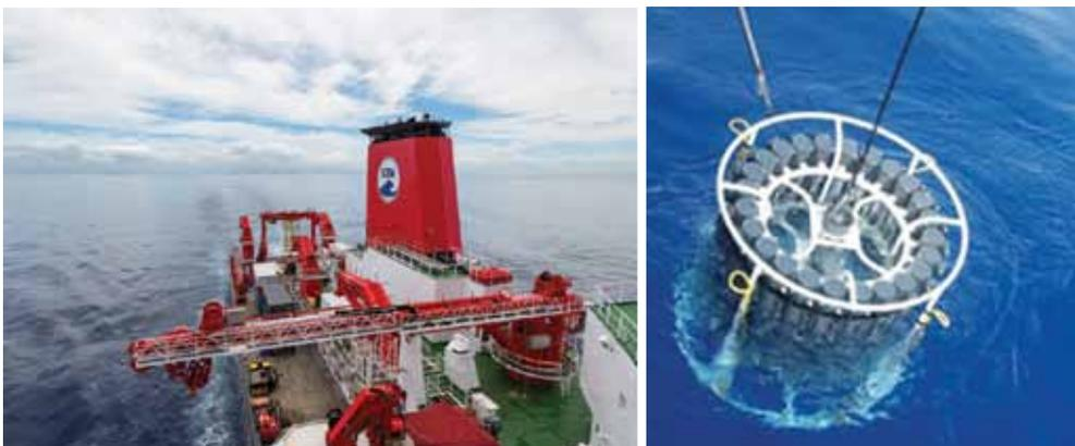
Figure 2. (L) German Research Vessel *Sonne*; (R) Trace metal clean rosette to collect trace metal clean water samples. Photographs: Nico Fröhberg (taken during the SO253 sampling campaign in 2017).
